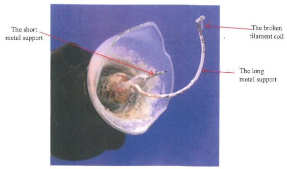
**Photograph 2:** The damaged light bulb (control light bulb obtained in the laboratory) before the in-house experiment.
