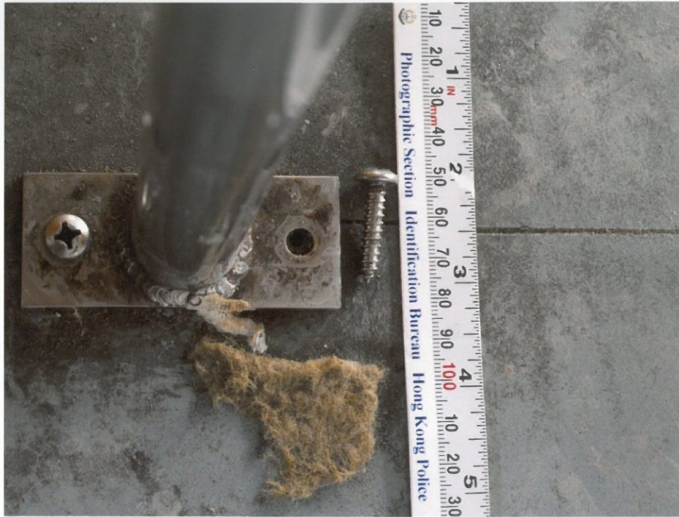
Photo 23: The rectangular mounting plate at the base of the leg of seat in the upper-deck cabin of Lamma IV and the screw for affixing the seat.
