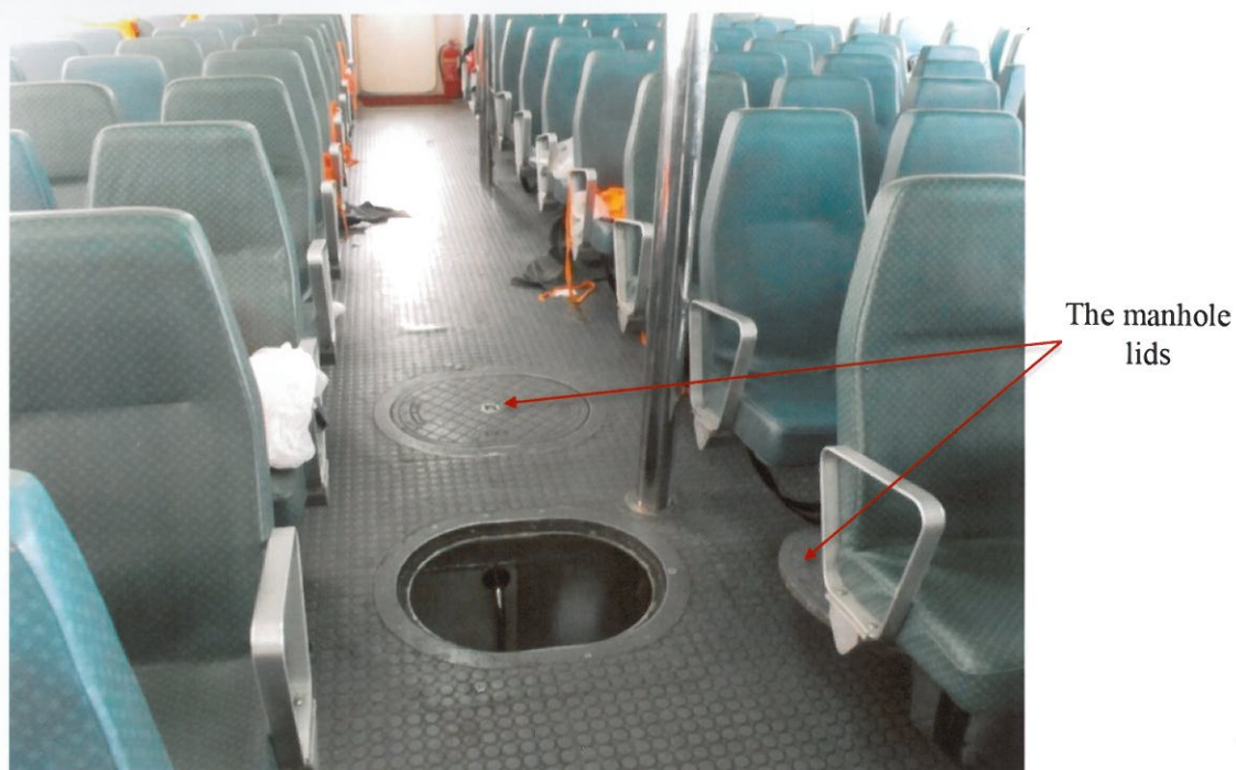
Photo 7: The manholes in the main-deck cabin of Sea Smooth access to Compartments 4 and 5 of the port hull.
