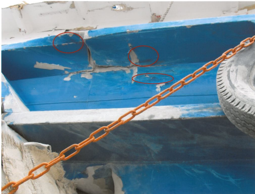
Photo 12: The horizontal scratches with deep blue smears (red circled) on the port side of the hull of Lamma IV
