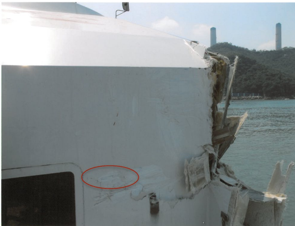
Photo 6: The blue smears (red circled) on the outer front panel of the main-deck cabin of Sea Smooth at the port side.
