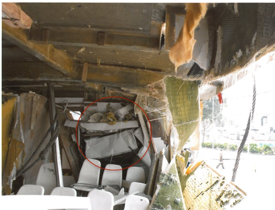
Photo 20: The crushed central unit of the air-conditioning system (red circled) and the collapsed seats at the port quarter of the main-deck cabin of Lamma IV
