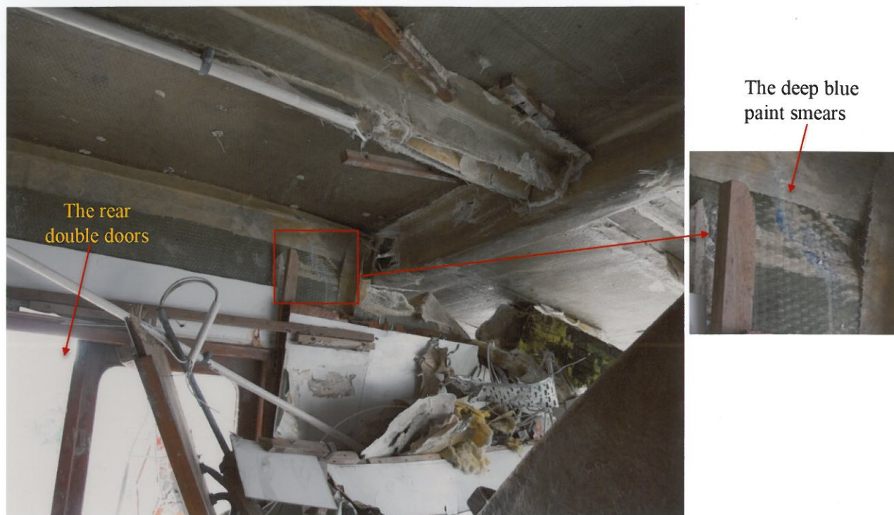
Photo 19: The deep blue paint smears found at the ceiling frame above the rear doors of the main-deck cabin of Lamma IV near the centreline
