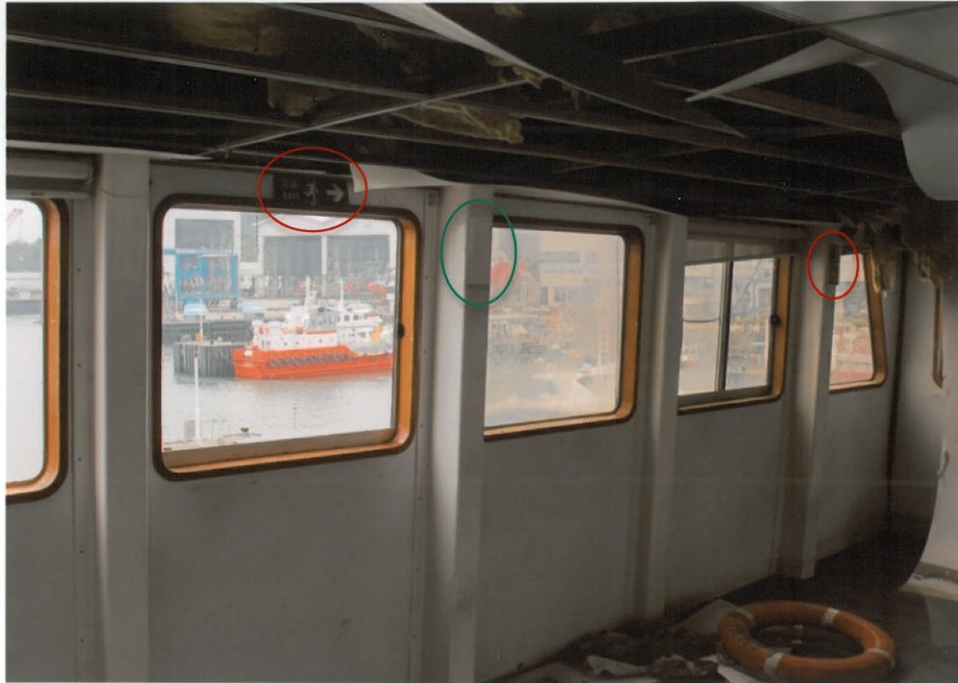
Photo 33: The exit signs (red circled) in the upper-deck cabin of Lamma IV. An imprint agreed in size with an exit sign (green circled).
