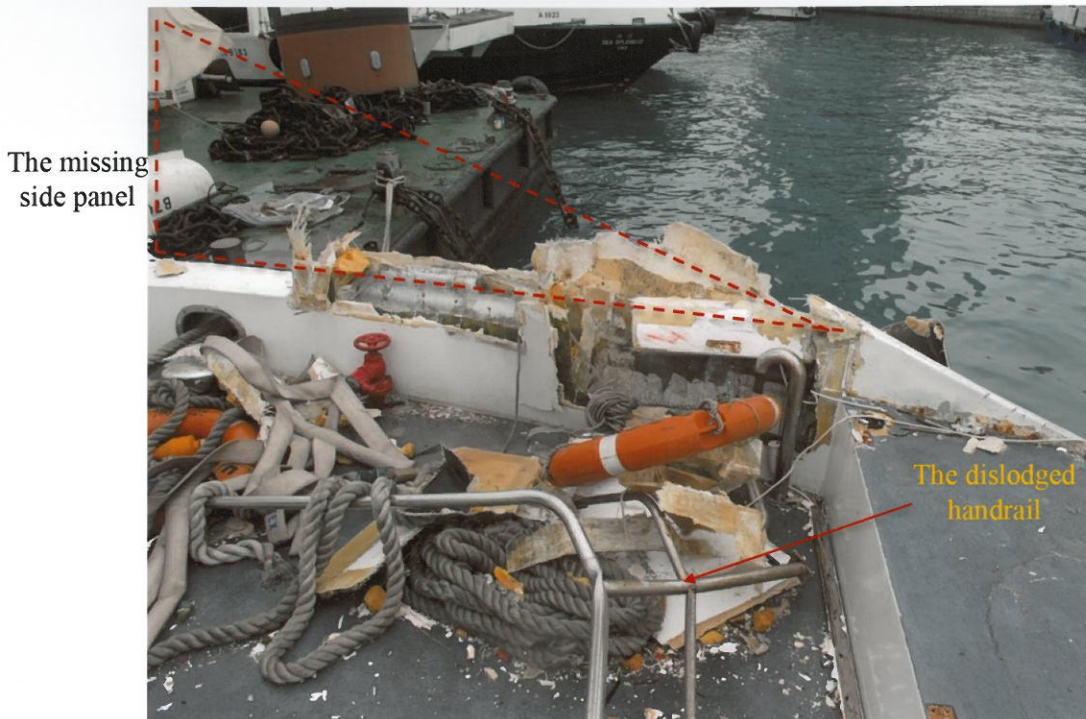
Photo 5: This showed the foredeck of Sea Smooth on the port bow. The side panel at the port bow was missing and the handrail was dislodged.
