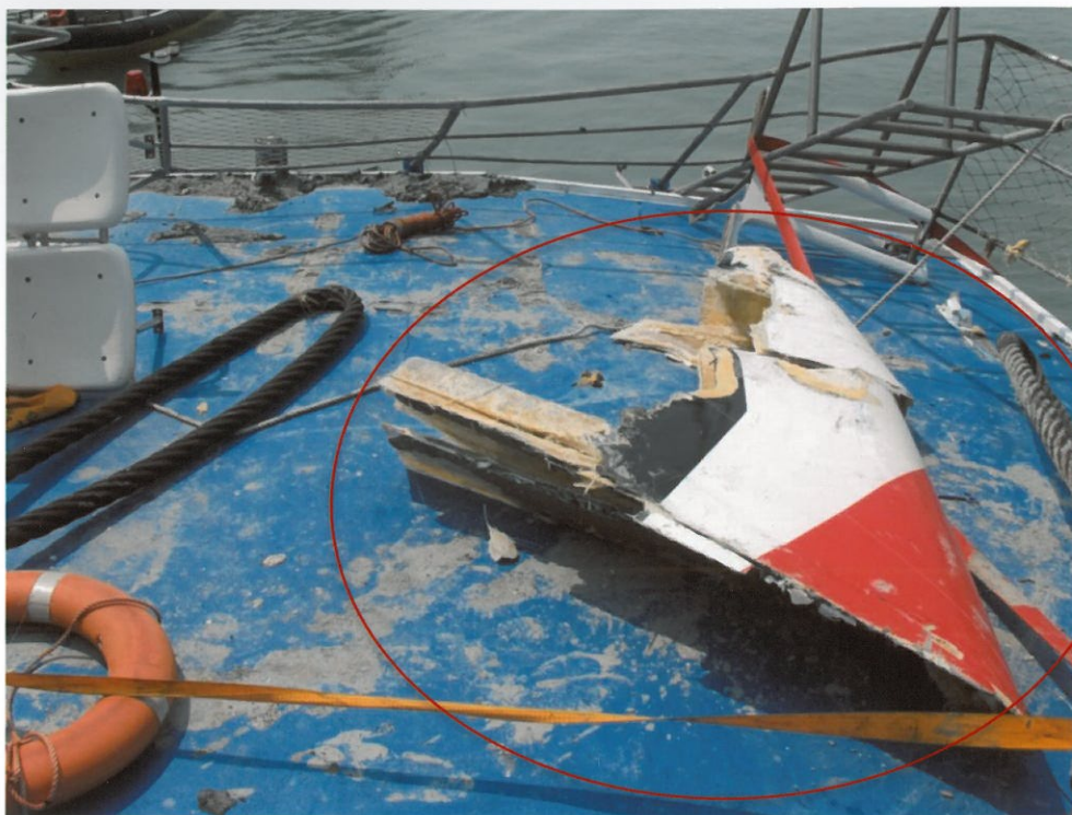
Photo 29: The piece of fibreboard fragment (red circled) on weather deck of Lamma IV
