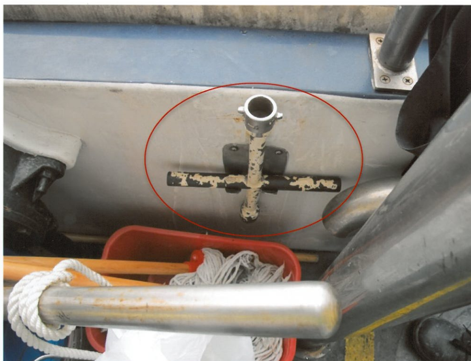
Photo 8: The cross wrench (red circled) at the stern of Sea Smooth for opening the manholes in the main-deck cabin for access to the compartments in the under deck.
