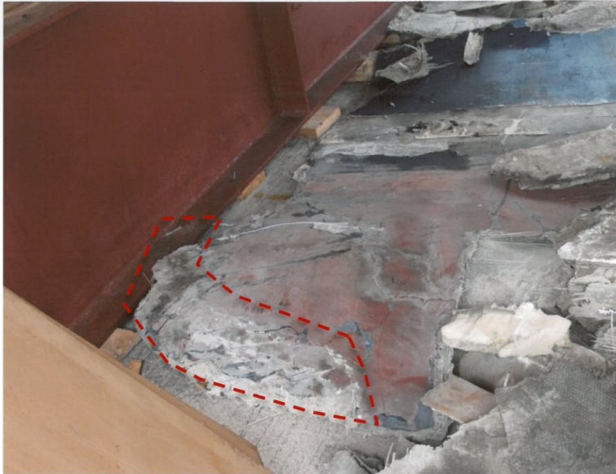
Photo 13: The imprint, marked by dotted line, on the fibreboard fragment belonging to the bow of the port hull of Sea Smooth
