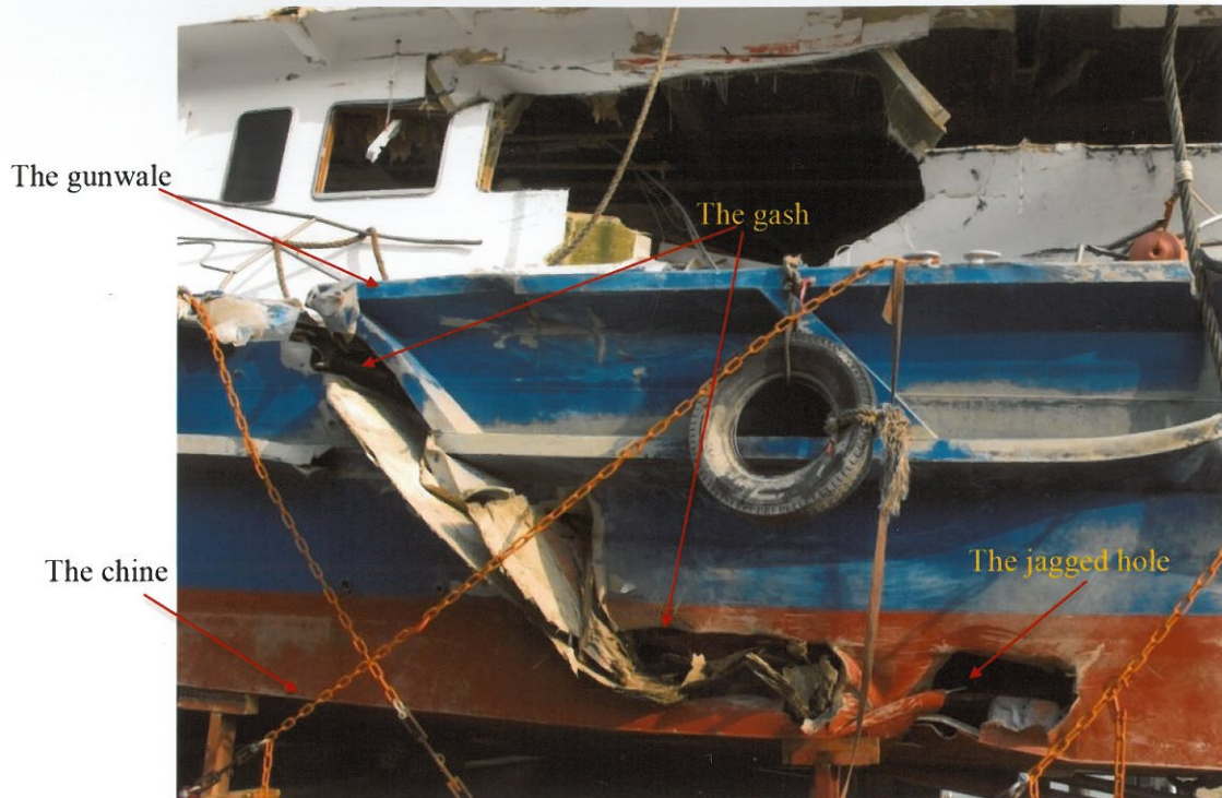
Photo 11: The gash and the jagged hole on the port side of the hull of Lamma IV
