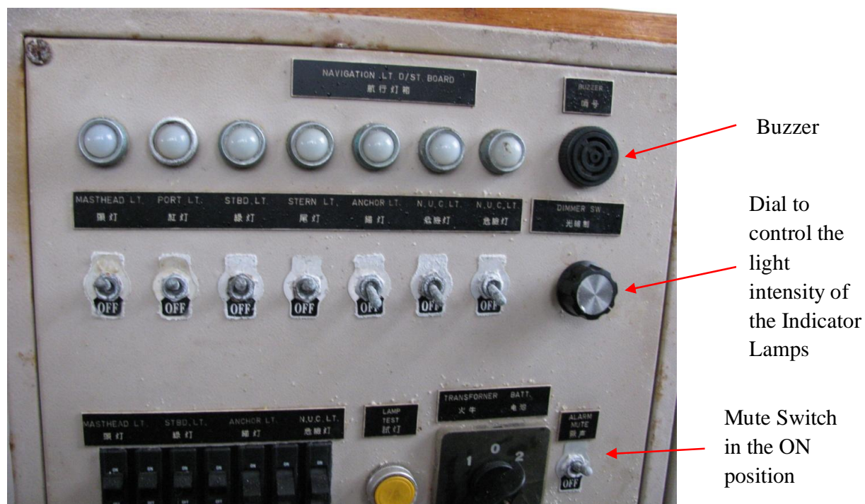
Photo 4 The intensity of the Indicator Lamps can be controlled by the dial as shown in the photo
