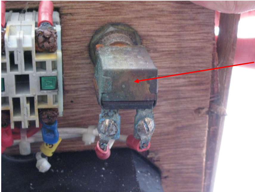
Photo 19 Rusts of copper oxide were observed on the switch associated with the ðHORNö button.
