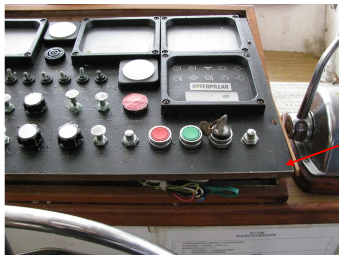
Photo 18 The controls of the various circuits, including the one marked with the description of "HORN". It is understood that by pressing the "HORN" button, a loud HORN would be produced to alert other vessels.
