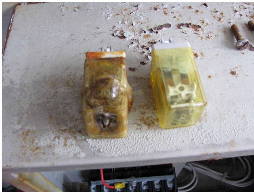
Photo 8 Another view of the disfigured relay and ðhealthyö relay. From the outside appearance of the dis-figured relay, one can confirm that high current had been flowing through the Coil inside the Relay for a prolonged period, of the order of at least several minutes. The reason for such high current was possibly because the devices in series with the Coil inside the Relay had been short-circuited.
