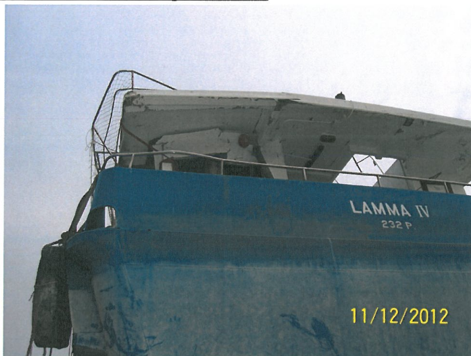
Appendix V – Photo 1. Stern view of Lamma IV illustrating limit of damage to the after end of the hull and superstructure
