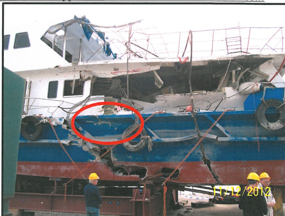
Appendix V – Photo 2. Lamma IV showing damage from collision bulkhead of Sea Smooth which stopped the forward momentum of Sea Smooth
